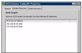
**10** If the connected ETERNUS DX Disk storage system uses multiple iSCSI ports, repeat the IP address addition process for each iSCSI port. (Repeat <a href="Step 7">Step 7</a> through <a href="Step 9">Step 9</a>.)
